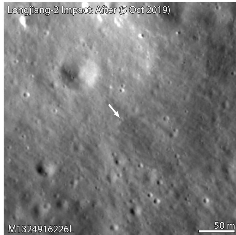
Figure 4.3: Crater created by the impact of 45 kg spacecraft Longjiang-2. Crater is 4 meters by 5 meters in diameter, seen from the LRO [69].
